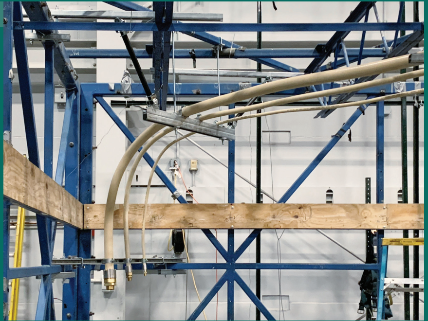
MediTrac® CMT in seismic test rig.
