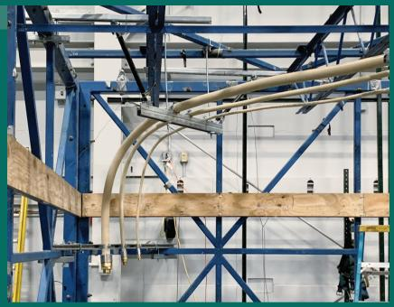
MediTrac® CMT in seismic test rig.
