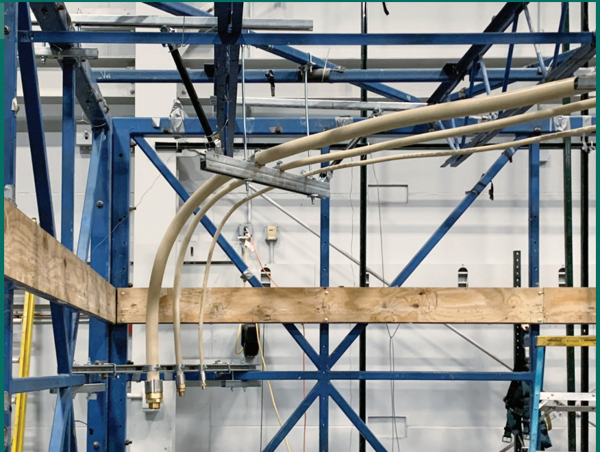
MediTrac® CMT in seismic test rig.
